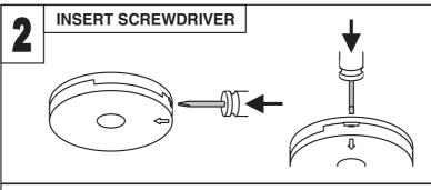
INSERT A FLAT-BLADED SCREWDRIVER HORIZONTALLY APPROX. 1cm INTO THE CENTRE OF THE REMOVAL SLOT
